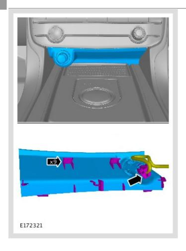
Remove the 12v accessory socket trim panel and disconnect the electrical connector.
