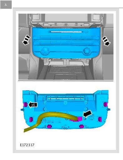
Remove the integrated control panel.
